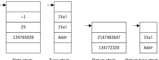
Data stack Type stack Return stack Return type stack Figure 1: The kForth Stacks The stack pointers are always aligned for each pair of stacks.
