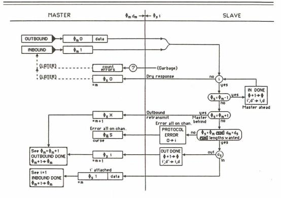
Figure 5a Logical Diagram of clusterFORTH Protocol
